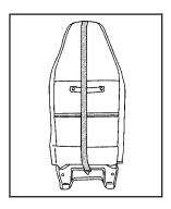
If the position you are using has an integrated headrest and you are using a single tether, route the tether over the headrest.
